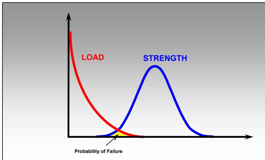
Figure 1. Illustration of Canonical Reliability Based Design
