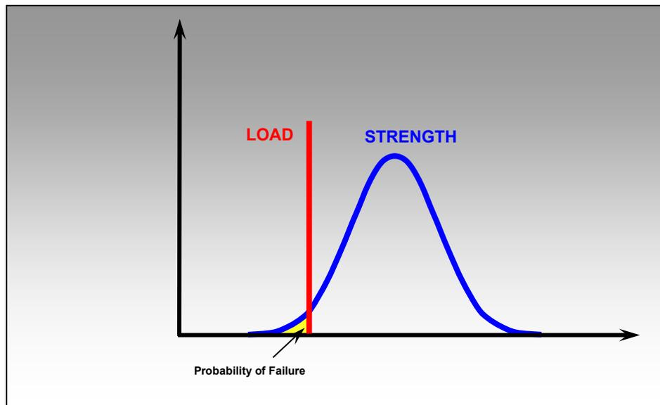
**Figure 2. Illustration of Deterministic Load and Probabilistic Strength (DLPS) Approach for Reliability-Based Pipeline Integrity Assessment**
