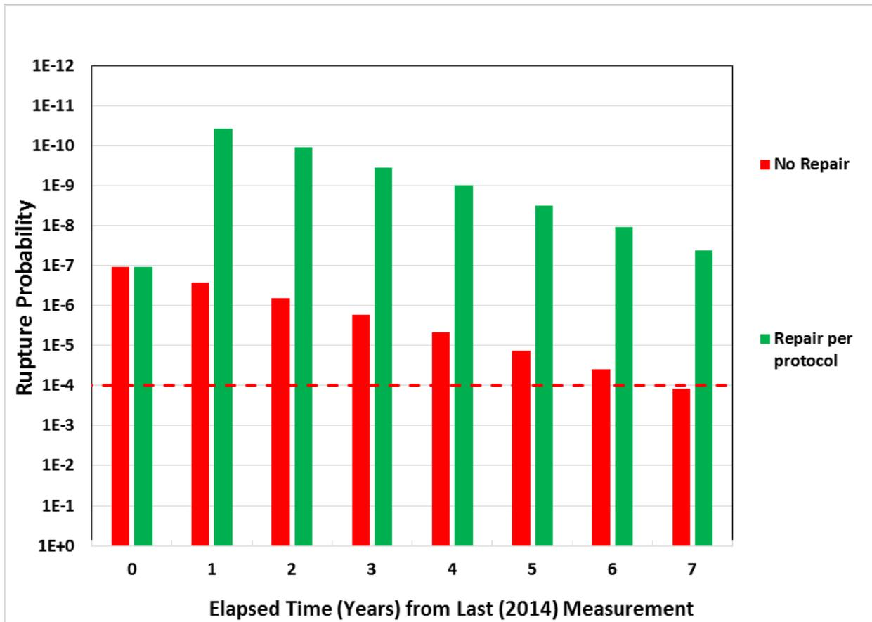
Figure 4. POF and SF for Class 3 Section as a Function of Time for Corrosion Anomalies – Both PHMSA and INGAA Protocols lead to the same outcomes and hence there is no distinction in the graphs
