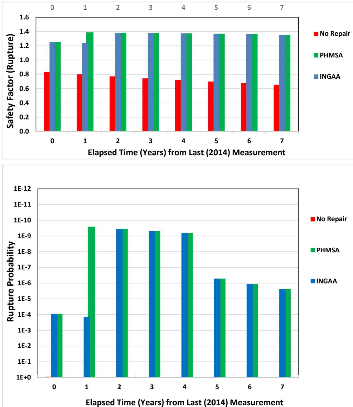
Figure 8: Comparison of SF and POF Changes with Time According to INGAA and PHMSA Protocols
