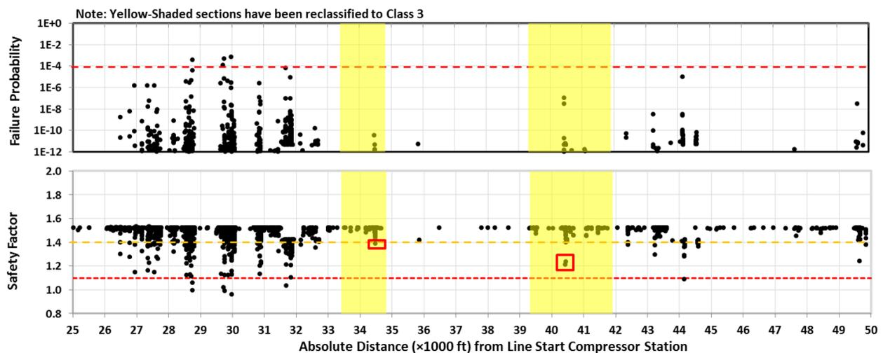
**Figure 3. Probability of Failure and Safety Factor Results for Pipeline Segment, Year Zero. Class change (1 to 3) locations are highlighted in yellow.**
