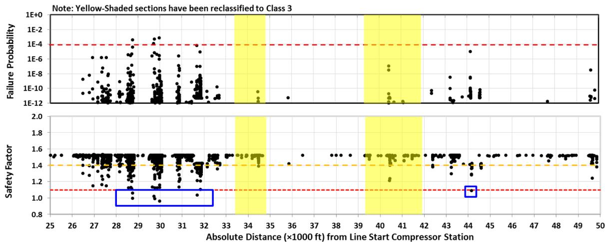
**Figure 7. Probability of Failure and Safety Factor Results for Pipeline Segment, Year Zero. Class 1 Anomalies Scheduled for Immediate Repair are Indicated.**
