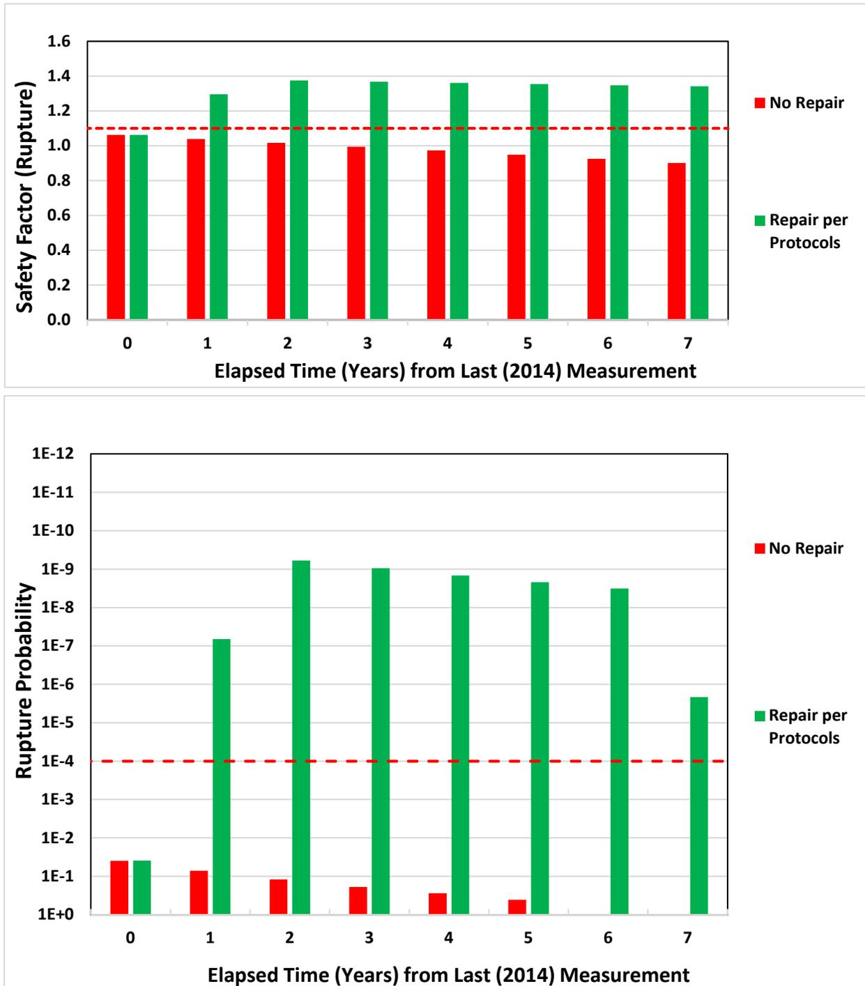
Figure 6. POF and SF for Class 3 Section as a Function of Time for SCC Anomalies – Both PHMSA and INGAA Protocols lead to the same outcomes and hence there is no distinction in the graphs
