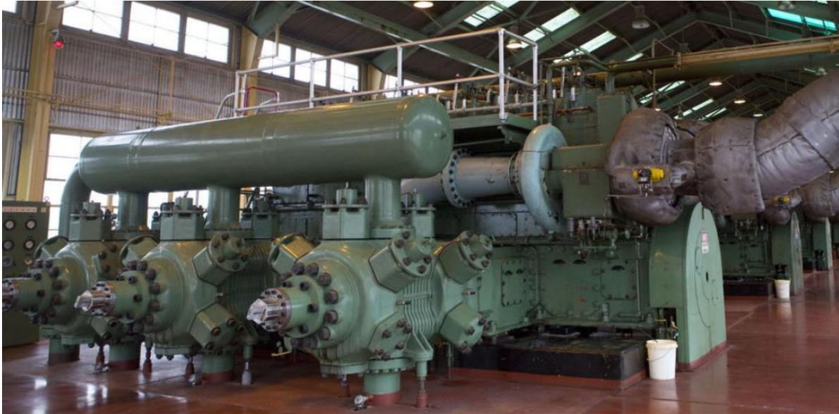
**Figure 3. Integral reciprocating compressors.**
