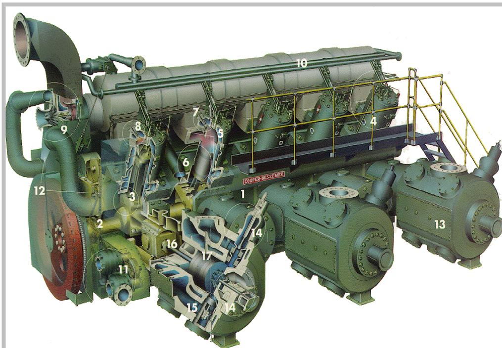
**Figure 4. Cutaway view of a Cooper Bessemer integral reciprocating compressor.**
