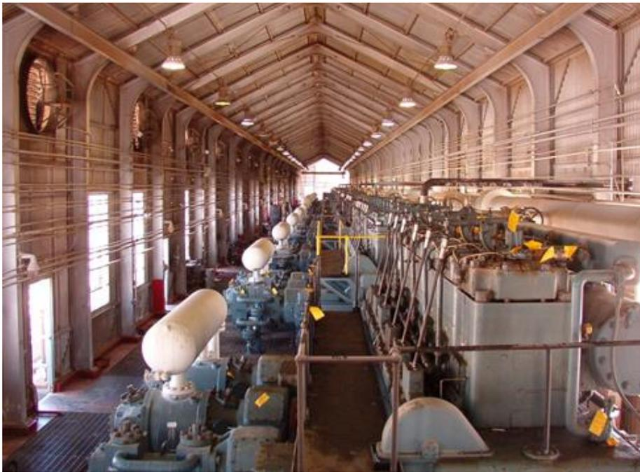
**Figure 1. Example of a compressor house (showing multiple integral reciprocating compressors).**
