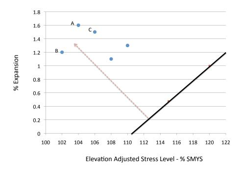
Figure 5 – Example Plot - Identification of Pipes With Expansion Levels Greater Than Predicted
