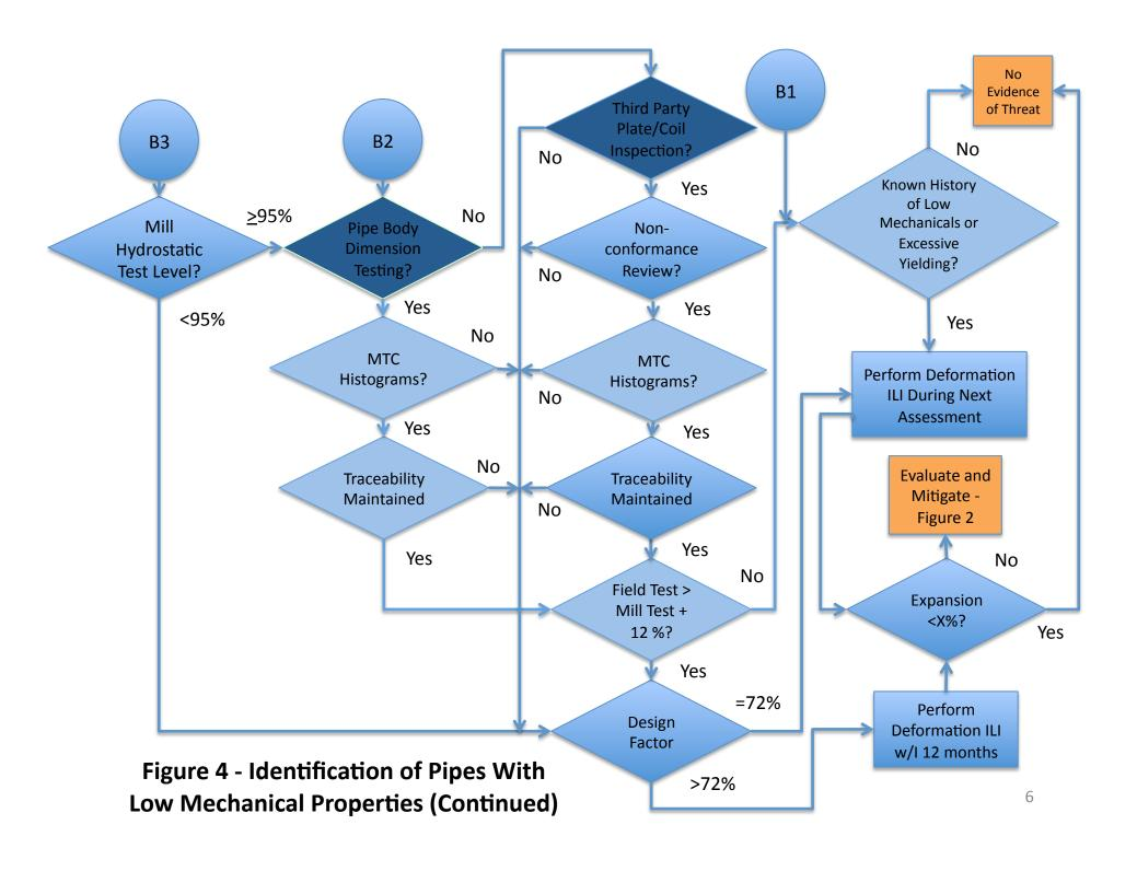
examination of information and records from the design, specification and manufacturing of the pipe to evaluate the potential for having expanded pipe. Figures 3 and 4 are provided for convenience so the reader can see how one moves from application of Figures 3 and 4 into the process being described in this white paper (depicted in Figure 2).
