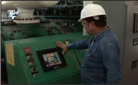
electric motor. One advantage of electric motors is that there is no need for an air emission permit, since no hydrocarbons are burned as fuel. Still, a highly reliable source of electric power must be available near the station for such units to be considered for an application.
