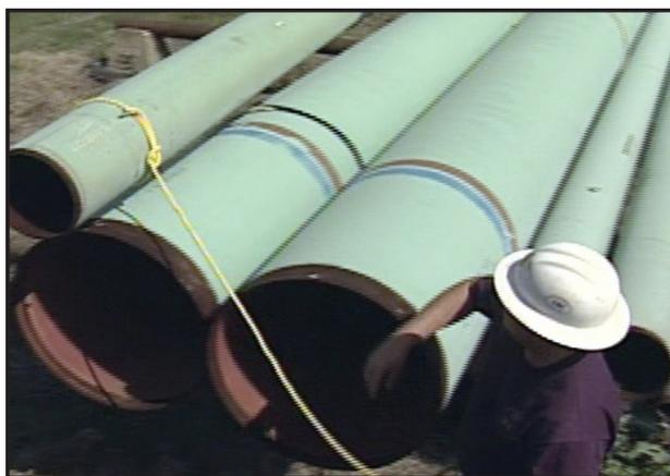
Seamless pipe is formed from a cylindrical bar of steel that is heated to a very high temperature and then is pierced with a probe to create the hole through the cylinder. Rollers size the cylinder to produce the proper diameter and wall thickness. This technique is used to make small diameter pipe, from 0.5 inches to 24 inches in diameter.
